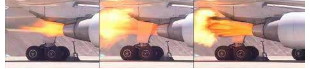
Resim 2: Tailpipe Fire ( https://www.infinidim.org/ )
